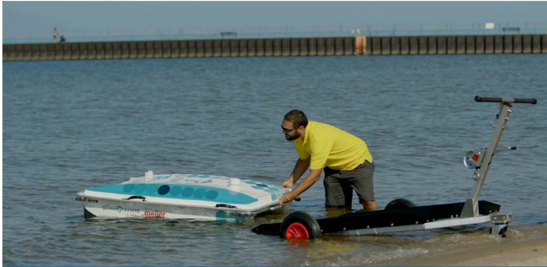
The Pixie Drone is a water drone built to collect up to 132 pounds of microplastics and other materials per use.
