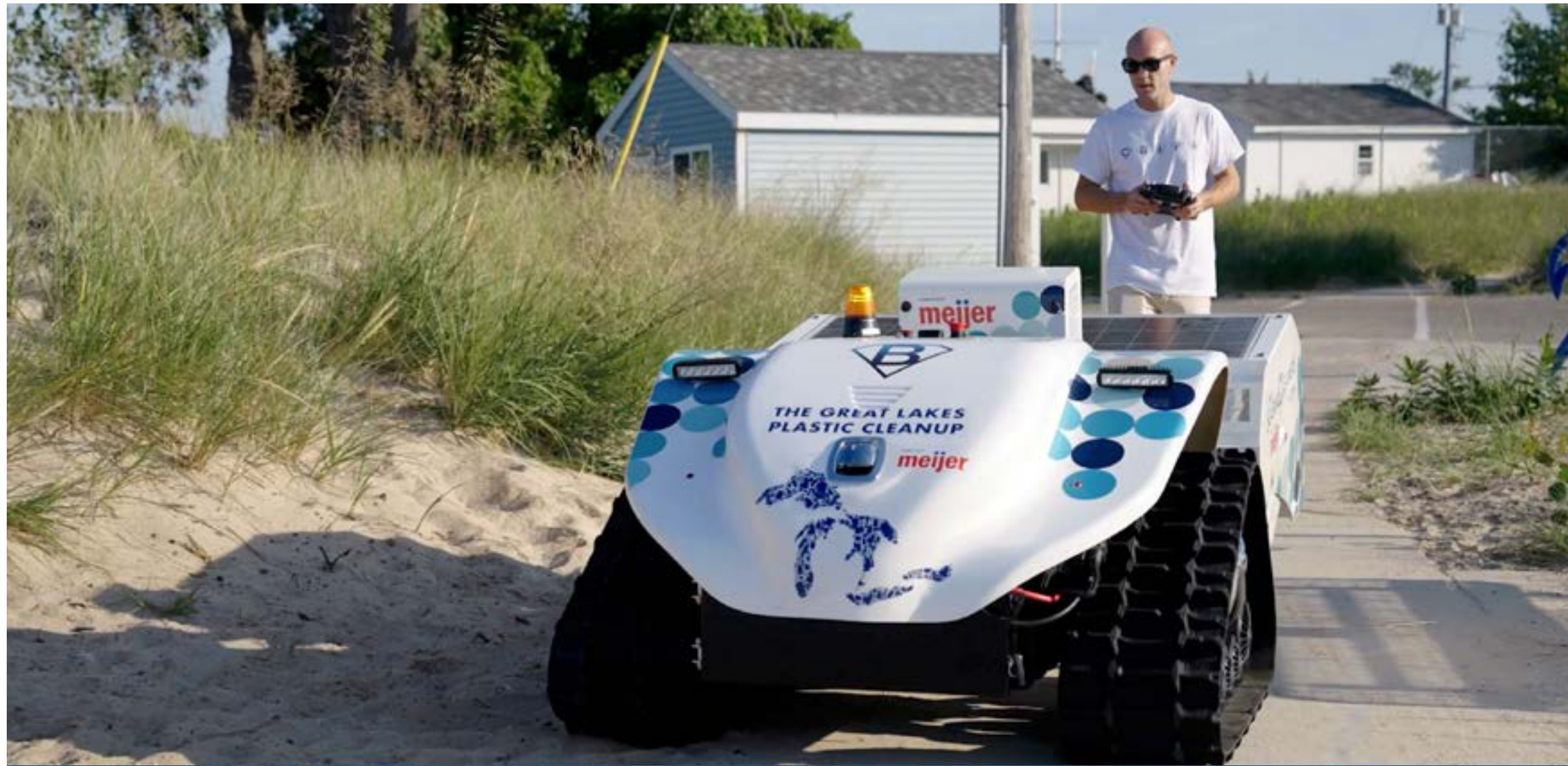
One BeBot can cover up to 32,000 square feet of lakefront beach per hour.
